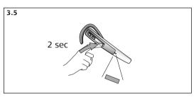
**3.5** Turn on headset by pressing Answer/End button for 1 sec. (visual indicator will flash blue four times and headset will beep three times), or by placing headset in charge cradle. Turn off headset by pressing Answer/End button for 2 sec. (visual indicator will flash blue four times and headset will beep three times).
